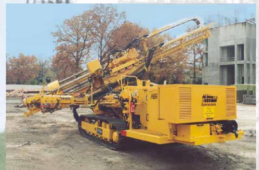
Mobile deep drill rigs, Hütte & Co.
